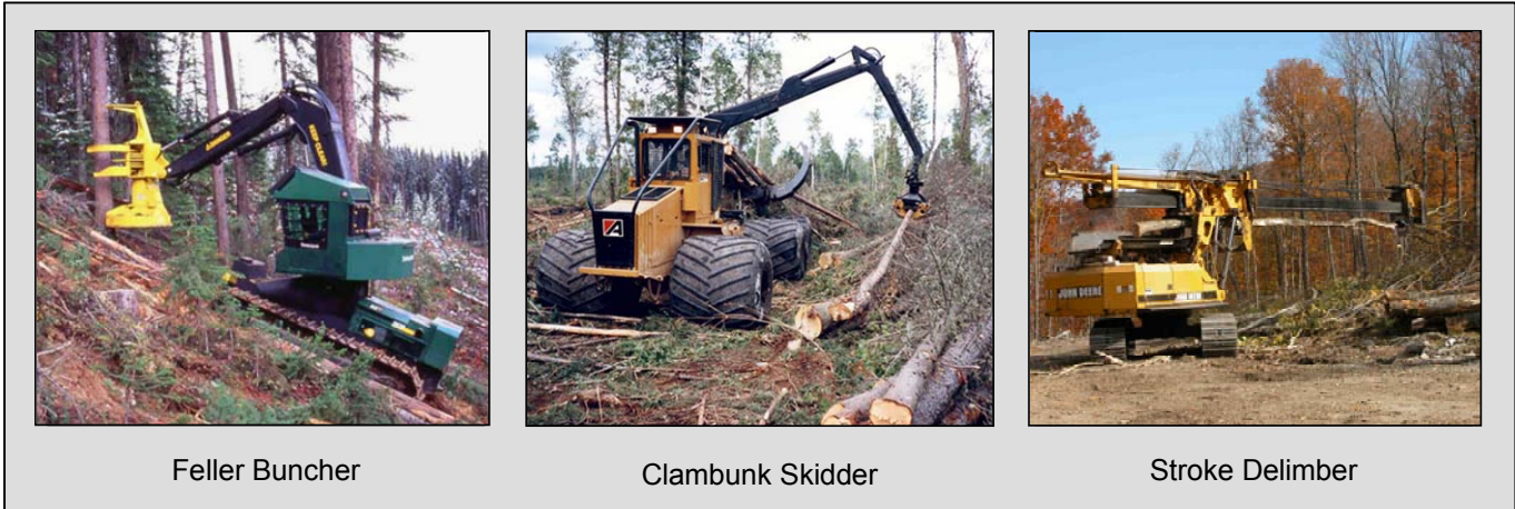
Figure 5: Non-Traditional Mechanical System Equipment 7
