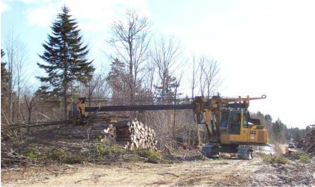
Figure 2: Stroke delimeter moving harvesting residue from the tree-length side of the landing to the harvesting residue side. 81
