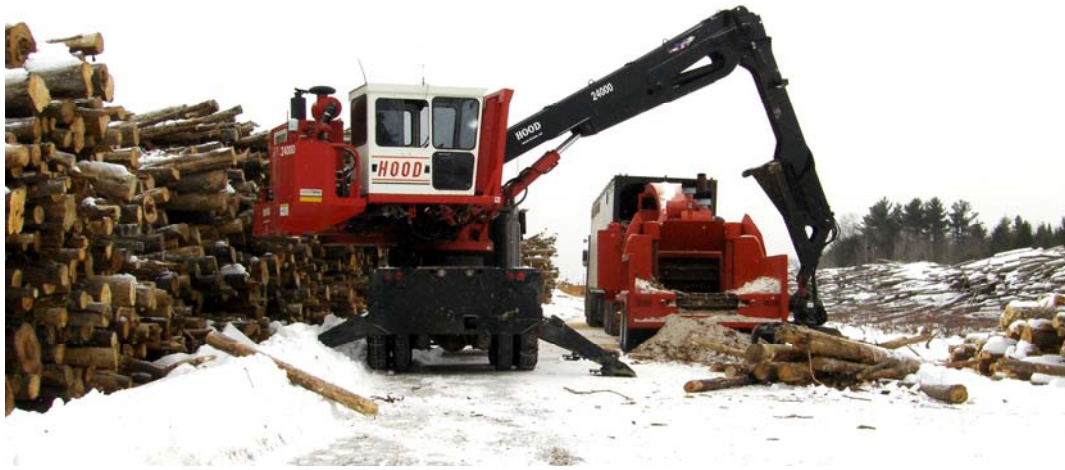
Figure 7: Processing harvesting residue into chips on a forest landing
