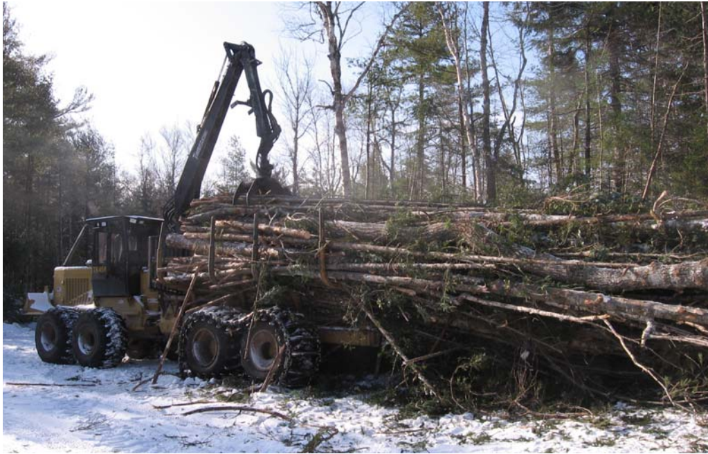
Figure 2: Forwarder moving biomass piles from the forest to the roadside landing
